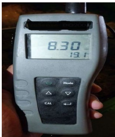
Photo 4: Digital multimeter for measuring oxygen (upper reading) and temperature (lower reading).
