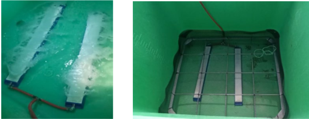
Photo 2: Oxygen diffusion ceramics installed inside the container and first-level rack, with red-coded hose (left side).
