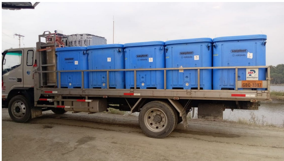
Photo 3: Flatbed truck loaded at the processing plant with prepared Saeplast insulated containers and liquid oxygen supply system.
