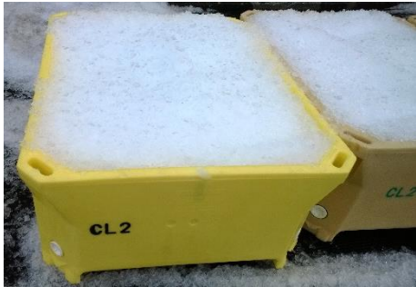
Figure 5. Sæplast 460 PUR (left) and Sæplast 460 PE (right) containers filled with ice at the beginning of an ice-melt test.
